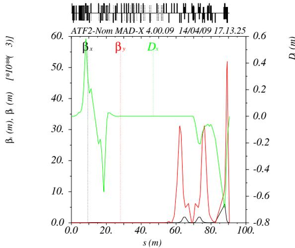
Figure 2: Nominal  $\beta_x$ ,  $\beta_y$  and horizontal Dispersion  $D_x$  functions for the ATF2 ultra-low  $\beta$  proposal. It should be noted the present symmetry around 70m concerning  $\beta_y$ .
