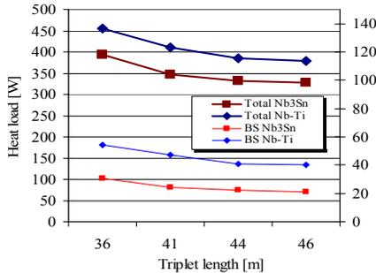
Figure 5: Total heat load on magnets, separating the contribution on the cold mass from the contribution on the beam screen, comparison between Nb-Ti and Nb<sub>3</sub>Sn layouts.
