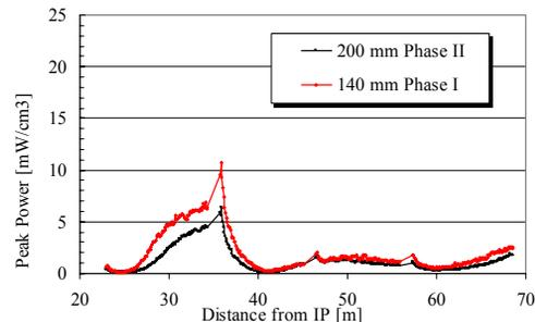
Figure 4: Peak power deposition in the coil for the 46 m long triplet, the case with a 140 mm Nb-Ti quad, and the case with 200 mm Nb<sub>3</sub>Sn quad, both cases without shielding for a peak luminosity of  $2.5 \times 10^{34}$  cm<sup>-2</sup> s<sup>-1</sup>.
