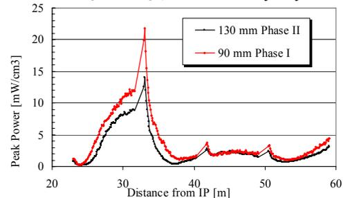
Figure 3: Peak power deposition in the coil for the 36 m long triplet, the case with a 90 mm Nb-Ti quad, and the case with 130 mm Nb<sub>3</sub>Sn quad, both cases without shielding for a peak luminosity of  $2.5 \times 10^{34}$  cm<sup>-2</sup> s<sup>-1</sup>.
