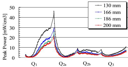
Figure 6: Peak power deposition in the coil for the four analysed lay-outs (Nb<sub>3</sub>Sn) for the luminosity  $10^{35} \text{ cm}^{-2} \text{ s}^{-1}$ , triplet length scaled to be the same for all layouts.
