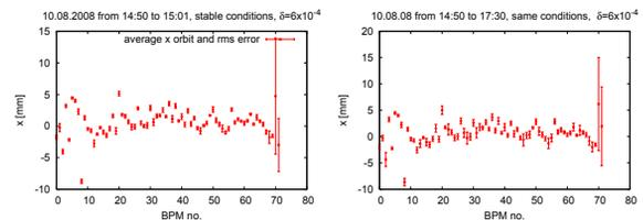
Figure 1: Average and rms reference trajectory in the horizontal plane computed from trajectory data taken over a 10-minute (left) and 3-hour interval (right) in the very first injection test on 10 August 2008.
