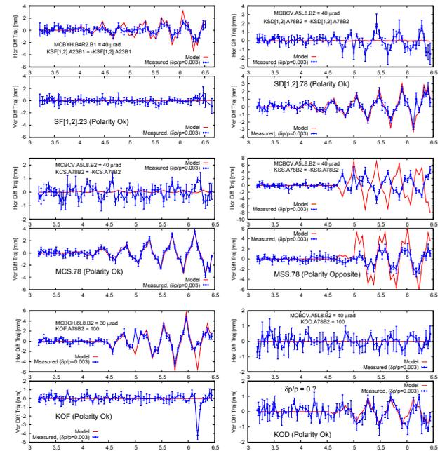
Figure 7: Difference of trajectories recorded at nominal and inverted strength for higher-order polarity checks compared with model predictions. Focusing (SF1&2.A23B2, top left) and defocusing lattice sextupoles (SD1&2.A78B2, top right). Sextupole spool-piece circuit (MCS.A78B2, center left). and skew-sextupole circuit (MSS.A78B2, center right). Focusing (ROF.A78.B2, bottom left) and defocusing Landau octupole circuit (ROD.A78.B2, bottom right). The orbit corrector polarities were also verified.
