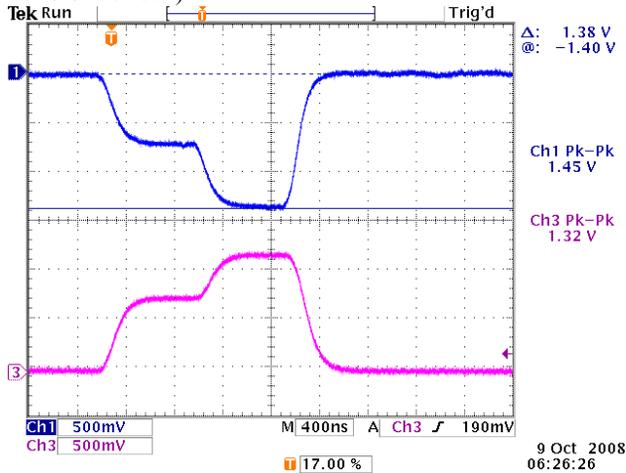
Figure 3: Electron current waveforms at the cathode (Ch1) and the collector (Ch3). Different polarity is due to the current transformer (CT) wiring. The CT calibration is 1 V/A.
