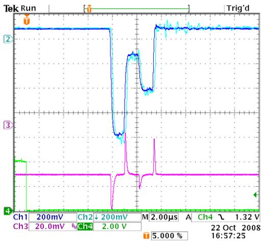
Figure 5: Example of an electron current waveform. Ch1 and Ch2 show the electron currents at the cathode and the collector. Ch3 shows the electron pulse as detected by a capacitive pickup.
