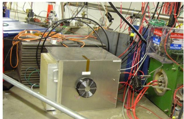
Figure 2: A photograph of the Stacked Transformer Modulator connected to the TEL2 electron gun in the Tevatron tunnel. The green magnet is the TEL2 gun solenoid.
