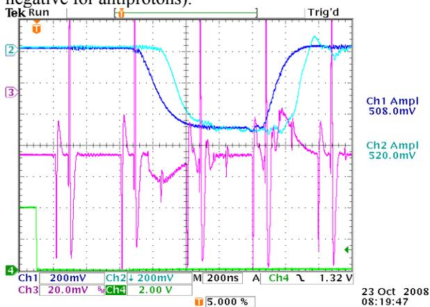
Figure 6: Electron pulse set up for two-bunch tune shift. Ch1 and Ch2 show the electron currents at the cathode and the collector. Ch3 shows the electron pulse and the antiproton and proton bunches as detected by the pickup. For clarity the pickup signal bandwidth is limited to 20 MHz.
