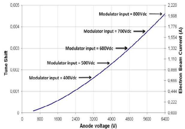
Figure 1: Required anode voltage for a given electron current and tune shift assuming standard TEL2 settings.
