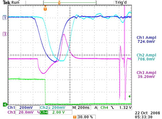
Figure 4: Electron pulse set up for a single bunch tune shift. Ch1 and Ch2 show the electron currents at the cathode and the collector. Ch3 shows the electron pulse, an antiproton bunch and a proton bunch as detected by a capacitive pickup. For clarity the electron pulse is timed to the abort gap and the pickup signal bandwidth is limited to 20 MHz.
