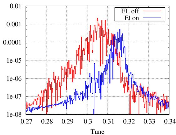
Figure 6: Vertical Shottky spectra with e-lens on (full compensation) and off. Total beam-beam tune shift  $\xi = 0.03$ .
