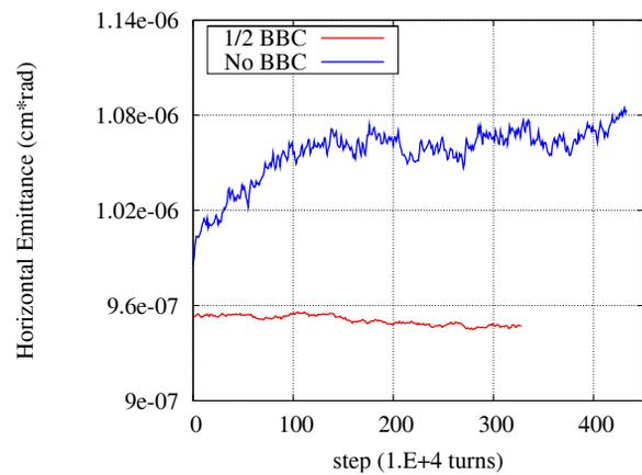
Figure 3: Horizontal beam emittance in RHIC with e-lens on (50% compensation) and off.  $\xi = 0.02$ .
