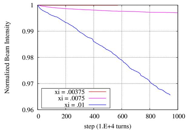
Figure 4: LHC beam life time for different values of beam-beam parameter per IP without beam-beam compensation.
