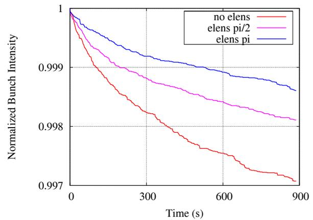
Figure 7: Effect of the phase advance between IP1 and the e-lens on the LHC beam life time.  $\xi = 0.03$ .
