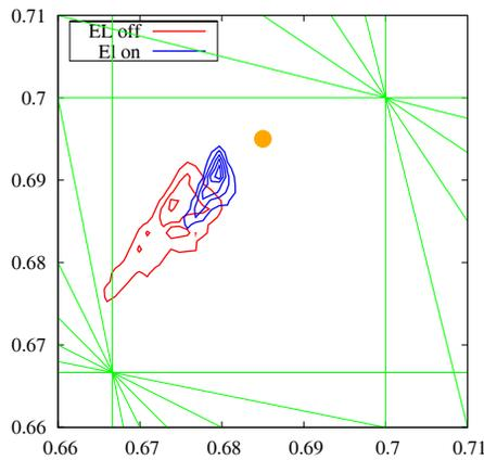
Figure 1: Tune footprint for RHIC with e-lens on (50% compensation) and off.  $\xi = 0.02$ .
