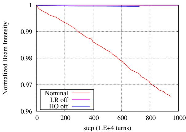
Figure 5: LHC beam life time with long-range (LR) and head-on (HO) collisions switched off.  $\xi = 0.04$ .
