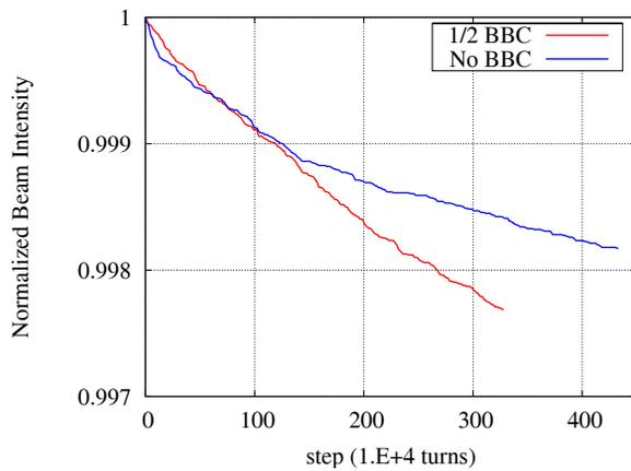
Figure 2: Beam life time in RHIC with e-lens on (50% compensation) and off.  $\xi = 0.02$ .
