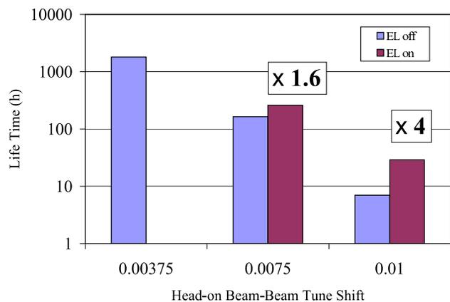
Figure 8: LHC beam life time for different values of beam-beam parameter with e-lens on (100% compensation) and off. The quoted value of beam-beam parameter is per IP (1/4).
