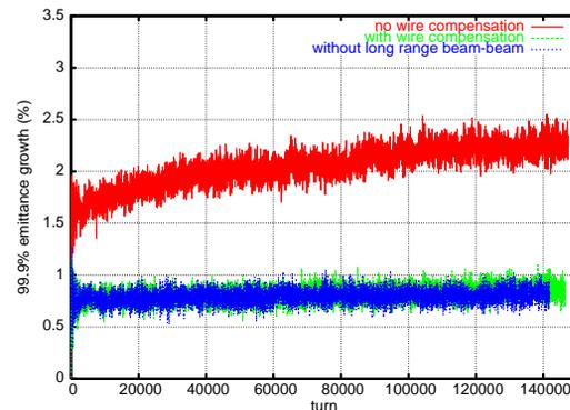
Figure 3: Emittance growth with/without wire compensation and the results without including long-range beam-beam effects.
