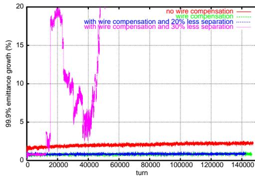
Figure 4: Emittance growth with/without wire compensation, with 20% reduction of nominal separation, and with 30% reduction of nominal separation.
