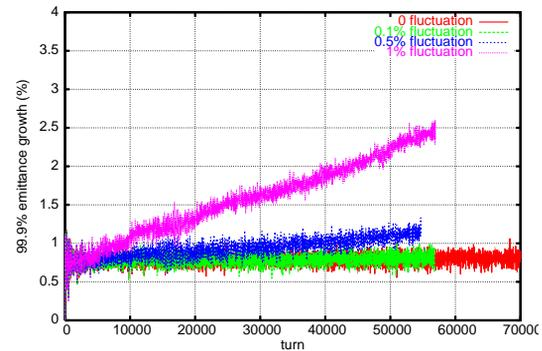
Figure 6: Emittance growth without current fluctuation, with 0.1%, 0.5%, and 1% current fluctuation.
