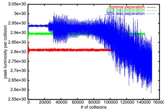
Figure 5: Peak luminosity evolution with nominal  $9\sigma$  separation, with 20% reduction of nominal separation, and with 30% reduction of nominal separation.
