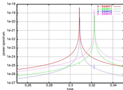
Figure 2: LHC betatron tunes from the BeamBeam3D simulation using a linear transfer map without beam-beam effects.
