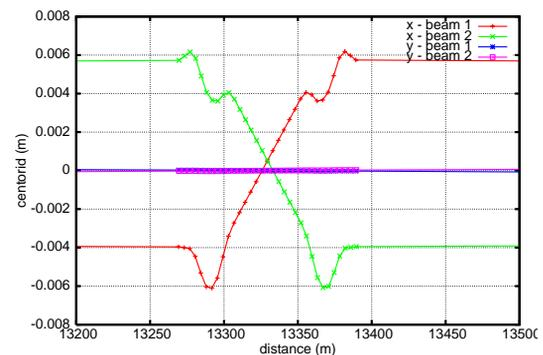
Figure 1: LHC beam-beam separation at IP IP 5.
