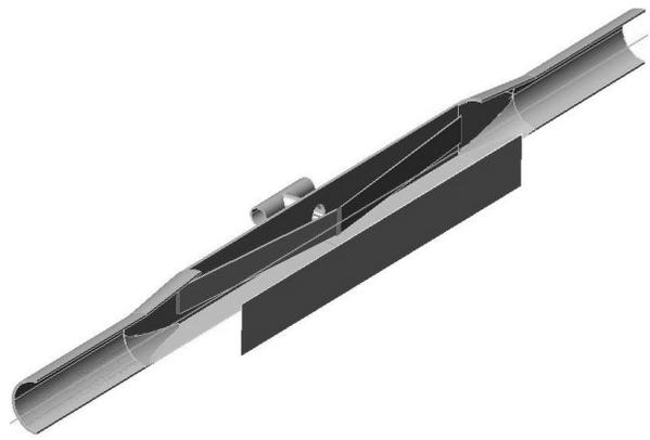
Figure 5: Photon stop to intercept synchrotron radiation at room temperature insertion between dipoles.
