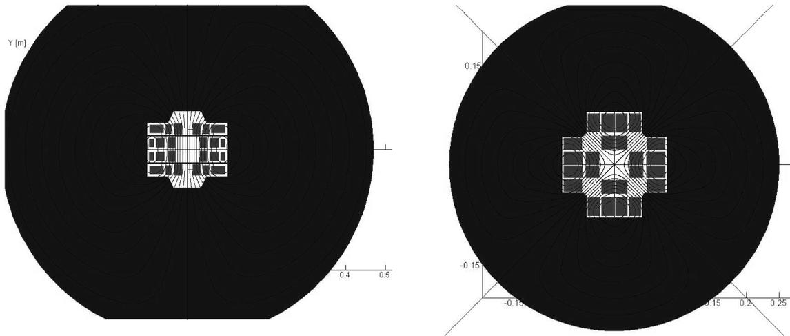
Figure 2: Cross sections of preliminary designs for 16.5 T dipole and 450 T/m quadrupole for 100 TeV collider.
