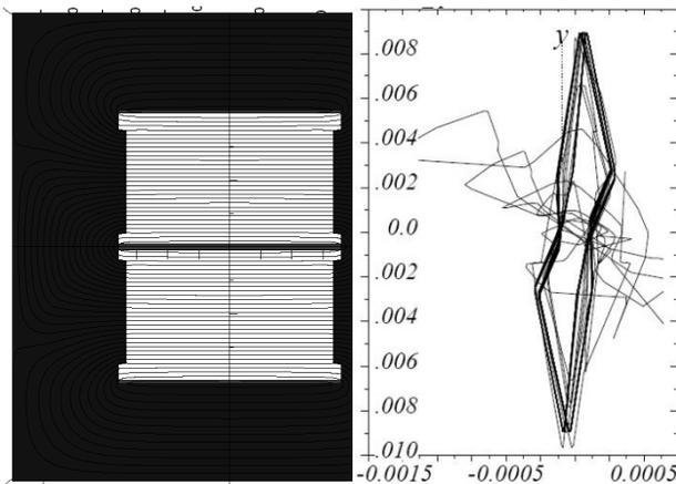
Figure 4: Vertical pretzel separation of beams: a) 1 T thin-septum dipole; b) separated orbits around the lattice.
