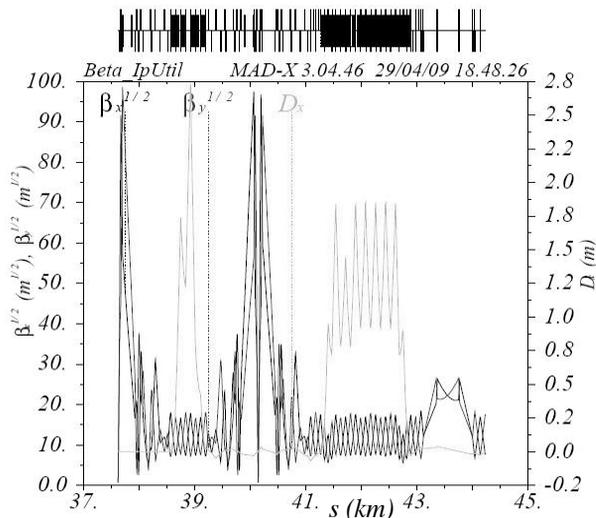
Figure 3: Lattice functions of Petavac, showing two low-beta insertions, dispersion matching, and one utility cell.
