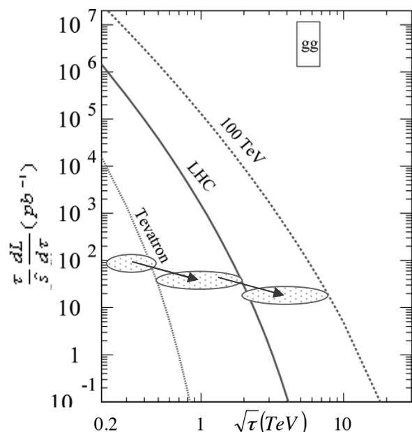
Figure 1: Parton luminosity vs. parton collision energy  $\sqrt{\tau}$  for the  $gg$  channel in Tevatron, LHC, and Petavac.
