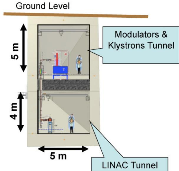
Figure 6: LINAC and Klystrons tunnel cross section.
