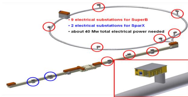
Figure 5: Electrical substations distribution.
