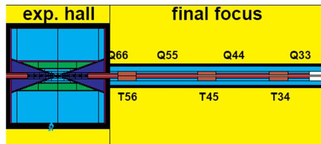
Figure 1: Sketch of the IP region and 130 meters of the final focus magnet system with quadrupoles (Q) and toroids (T). This sketch shows the geometry of the detector used in the 1996 GEANT simulation of a  $2 \times 2$  TeV Muon Collider. The conical tungsten-filled region, shown in dark blue, was required to absorb debris from muon decays in the beams. Because of the limitations of detector technology at the time, this area was not instrumented.
