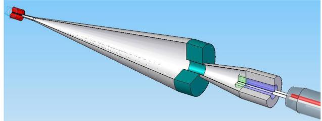
Figure 2: Illustration of conceptual forward calorimeters for luminosity (40-140 mr, shown in teal) and beam diagnostic (<40 mr, shown in blue) measurements. Advances in electronics that allow these designs can be used in a muon collider detector.
