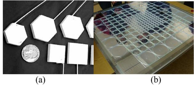
Figure 3 (a): Examples of plastic scintillator tiles for use in calorimeters made by the NIU group; (b): Array of scintillating tiles arranged on 1m x 1m plate of a prototype CALICE hadron calorimeter. The tiles are arranged as a mosaic with smaller tiles in the high rate regions and larger tiles farther away.
