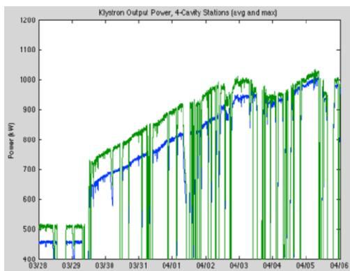
Figure 4: Plot of the klystron output power for the 4 cavity stations. The blue line is the average and the green line is the maximum during the time of the energy scan. Several klystrons were delivering 1 MW of output power.
