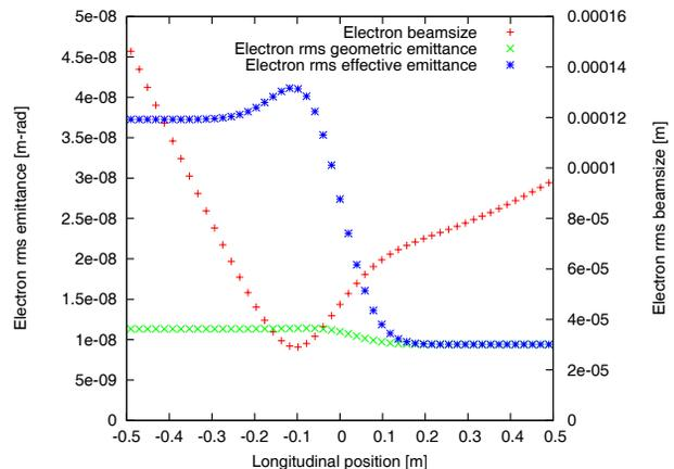
Figure 1: Electron beam evolution during beam-beam interaction.
