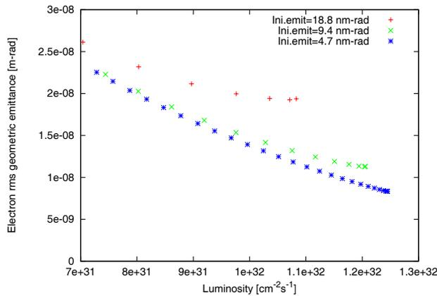
Figure 2: rms geometric emittance after collision as a function of the final luminosity. Each point corresponds to one initial electron emittance and design optics.
