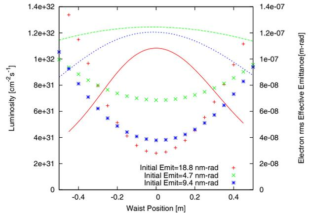
Figure 3: Luminosity and rms effective emittance as a function of the electron beam waist position.
