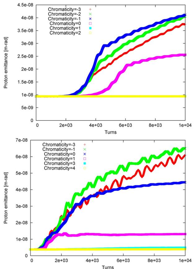
Figure 5: Proton emittance growth and suppression with chromaticity. Top: 'not-cooled case'; bottom: 'pre-cooled case'.
