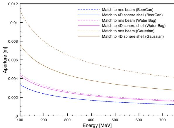
Figure 4: Apertures for zero beam loss at 100MeV to 750 MeV. Apertures of other energies can be scaled by inverse square root of the energy.
