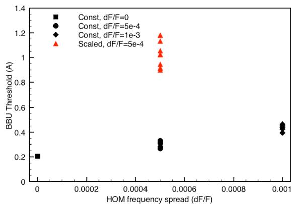
Figure 1: Simulated BBU threshold versus HOM frequency spread. Results are shown for constant gradient and scaled gradient variants of the linac optics.
