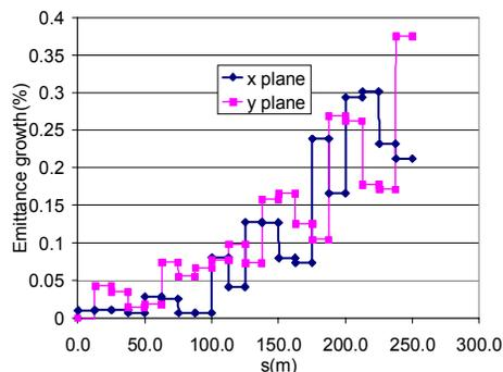
Figure 3. Emittance growth due to energy spread only
