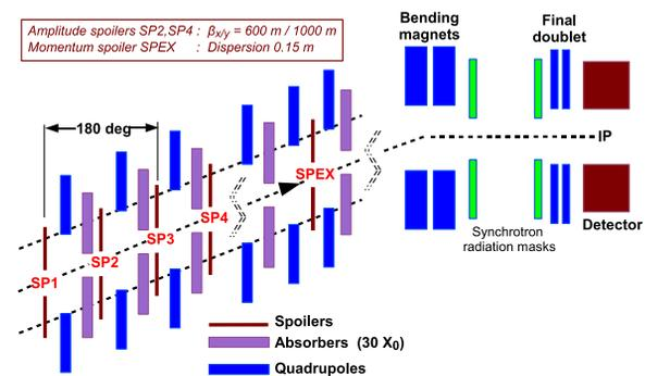
Figure 1: Layout of the ILC Beam Delivery System [2]. Shown are the amplitude spoilers SP1 to SP4 and the energy spoiler SPEX, which are due to their small apertures the critical components in case of magnet and klystron failures.
