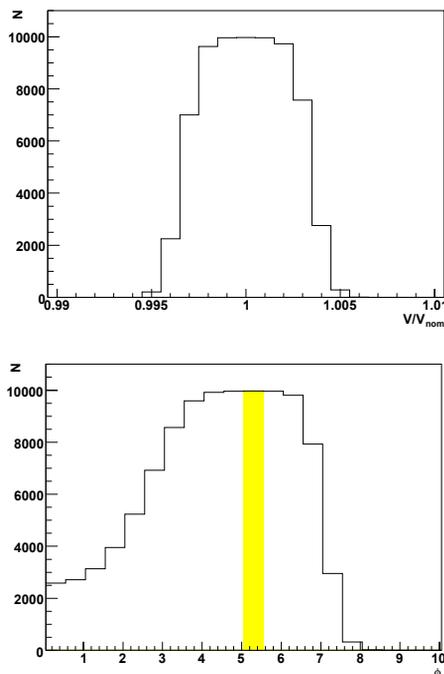
Figure 2: The upper plot shows the number of particles  $N$  reaching the interaction point vs. the relative voltage shift. The lower plot shows  $N$  vs. the phase shift in degrees. The band indicates the nominal phase. The shapes of the plots are related by the  $\cos \phi$  dependency of the accelerating voltage ( $V = V_0 \cos \phi$ ).
