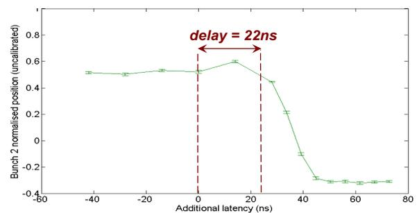
Figure 4: Kick to bunch 2 vs. added delay.
