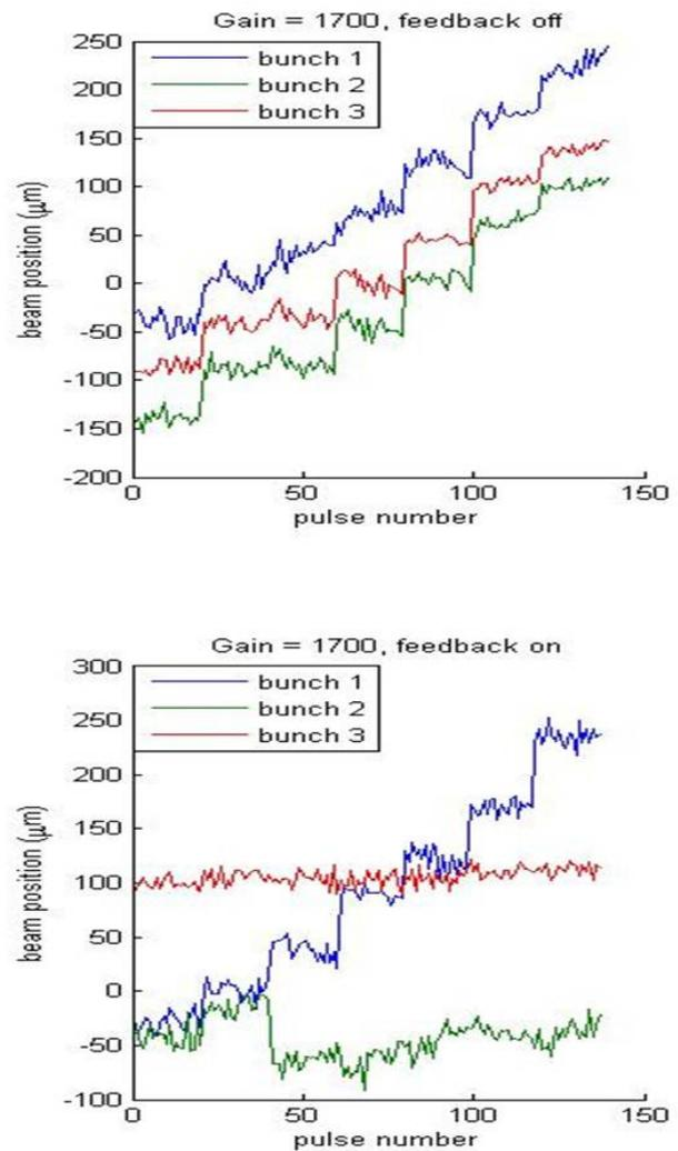
Figure 6: Beam position vs. pulse number: feedback off (top) and on (bottom).
