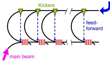
Fig. 3: Drive beam distribution system and PWFA cells.
