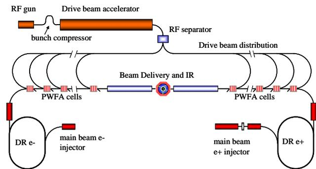
Fig. 1: Concept for a multi-stage PWFA Linear Collider.
