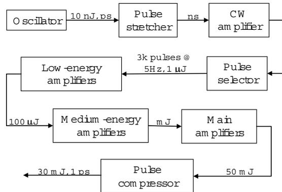
Figure 1: Block diagram of initial concept for the laser system.
