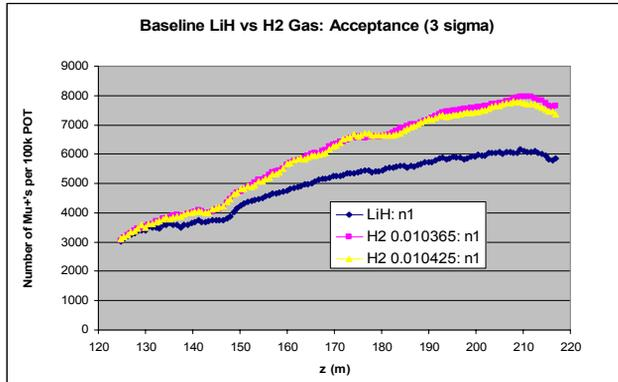
Figure 3. A comparison of muon capture with gas H<sub>2</sub> cooling or LiH cooling, as simulated using G4Beamline. The gas H<sub>2</sub> example obtains 33% more μ/p than the case with LiH cooling. H<sub>2</sub> density is 0.0104 gm/cm<sup>3</sup>.
