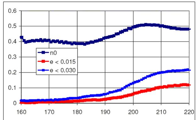
Figure 4: Capture of muons within the reference acceptances in the 24MV/m, 150atm H<sub>2</sub> case. The horizontal axis is distance along the transport in m. (The φ-E rotator cooler begins at z=163 and ends at z=217m.) The upper trace is total μ/p; the lower traces are μ/p in the acceptance of  $\epsilon_L < 0.15$ m,  $\epsilon_{\perp} < 0.03$ m and  $\epsilon_{\perp} < 0.015$ m.
