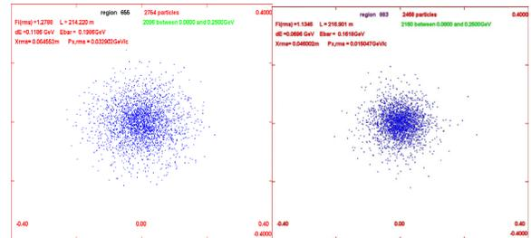
Figure 5. Transverse beam sizes in the front end after equivalent energy-loss LiH cooling(left) and after gaseous  $\text{H}_2$  cooling(right). (Horizontal and vertical axes are  $\pm 0.4\text{m}$ )
