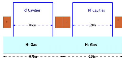
Figure 2: A cell of the gas-filled cooling system. (radial cross-section view) This contains 0.5m long "pillbox" 201.25 MHz rf cavities, with 0.25m gaps between cavities containing coils for magnetic fields. The  $H_2$  gas fills the center of the transport with a uniform density.
