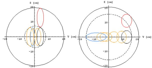
Figure 6: Aperture of normal (dashed circle) and special magnets (solid circle) defined by  $3\pi$  cm beam ellipses over momentum range for both the D (left) and F (right) magnets. The red ellipse represents the kicked beam.
