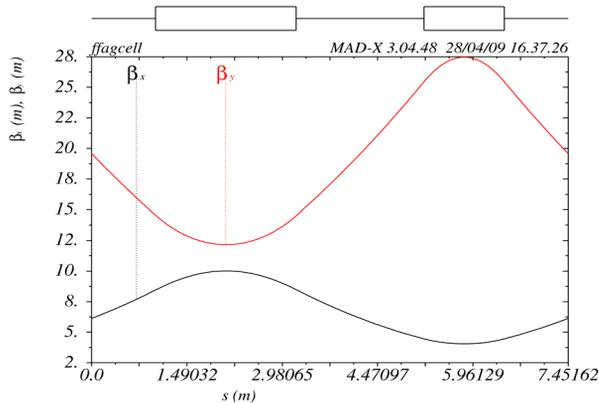
Figure 4: Betatron functions at extraction energy (25 GeV) in the FODO FFAG ring.
