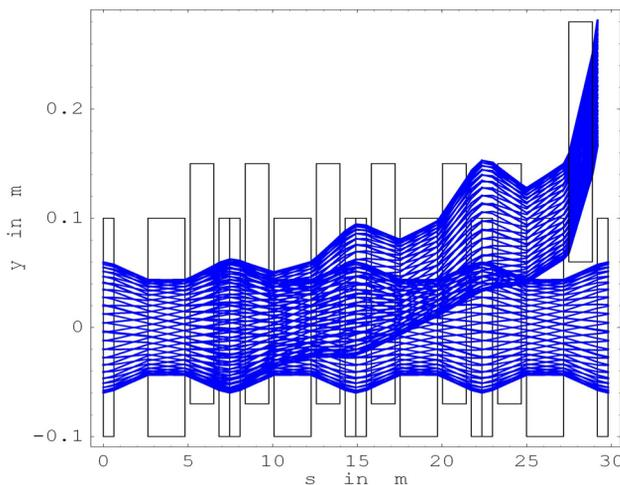
Figure 5: Vertical extraction scheme from the FODO FFAG ring using 6 kicker magnets.
