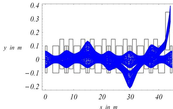
Figure 3: Vertical injection scheme into the FODO FFAG ring using 10 kicker magnets ( $5\pi/2$  betatron oscillations).
