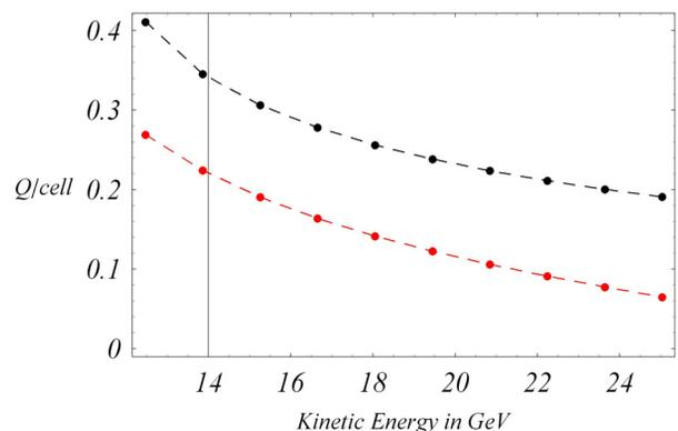
Figure 1: Tunes as a function of energy in the FODO FFAG ring. Dots correspond to Zgoubi [4] results and dashed lines to BeamOptics [5] ones (black is horizontal tune and red is the vertical one).
