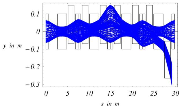
Figure 2: Vertical injection scheme into the FODO FFAG ring using 6 kicker magnets ( $3\pi/2$  betatron oscillations).
