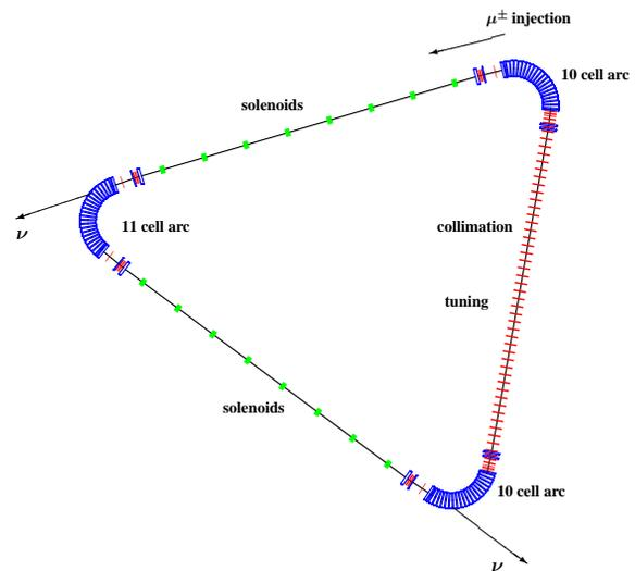
Figure 4: Layout of isosceles triangle ring
