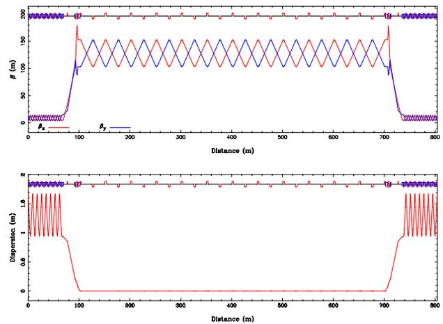
Figure 3: Optical functions for the racetrack ring
