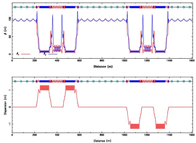
Figure 7: Optical functions of the bow-tie ring
