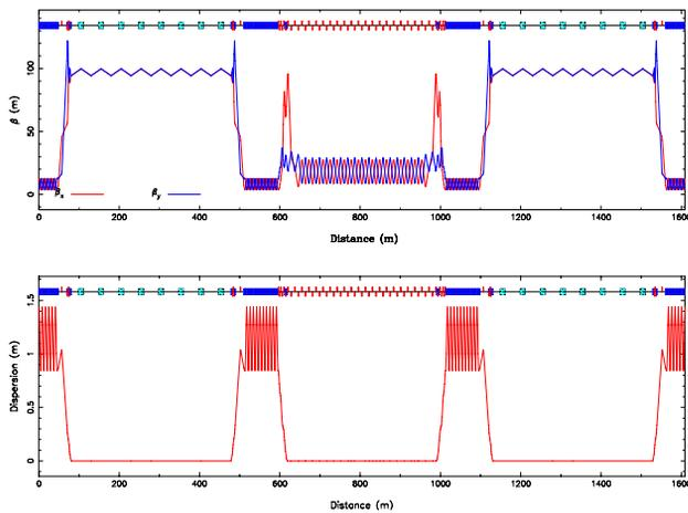
Figure 5: Optical functions of the isosceles ring
