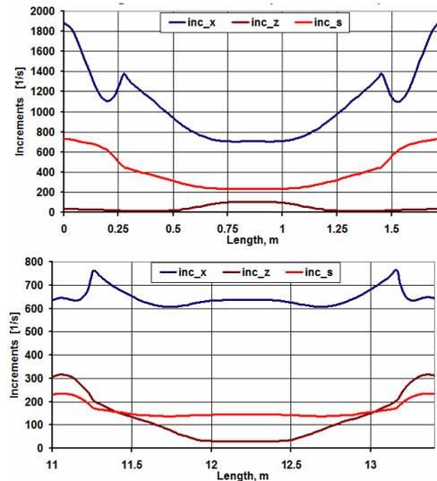
Figure 5: Horizontal (blue), vertical (brown) and longitudinal IBS growth rate increments for the original (top) and the modified TME cell (bottom).
