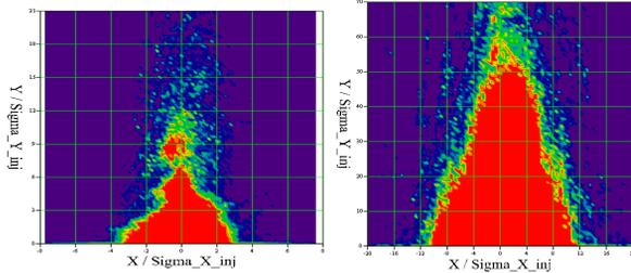
Figure 4: On-momentum DA for the original (left) and the modified DR (right).
