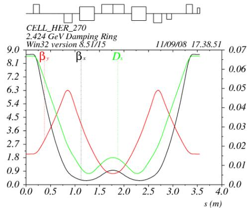
Figure 6: Alternative arc cell optics based on the SuperB ring cell.
