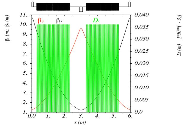
Figure 2: Optical functions (left) and geometry aperture (right) for the optimized FODO cell.
