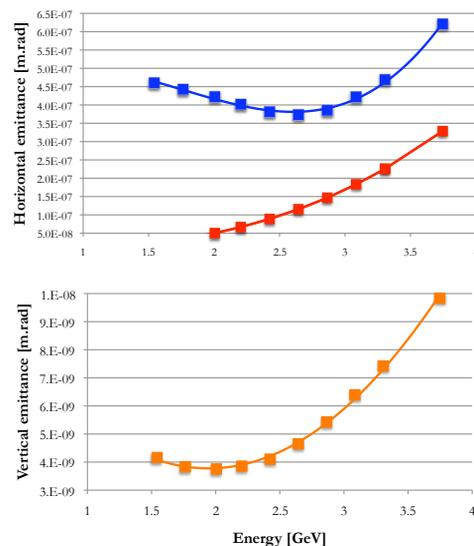
Figure 1: Horizontal normalized emittance (top) versus the energy, with (blue) and without the effect of IBS (red) and vertical normalized emittance (bottom).
