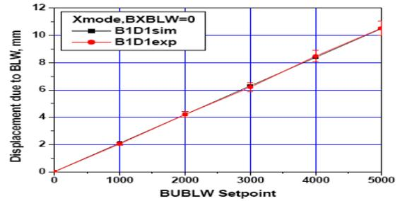
Figure 4: Maximum excursion of the difference orbit vs. BUBLW setpoint at B1D1PUE while BXBLW is OFF.
