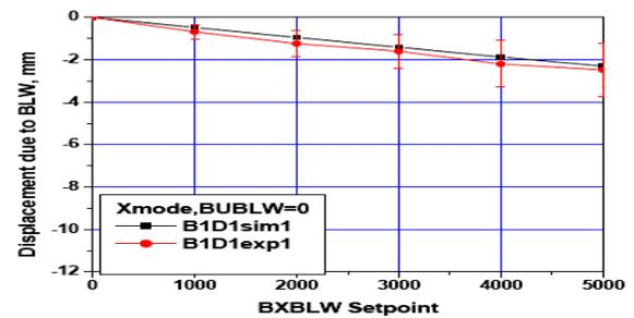
Figure 6: Maximum excursion of the difference orbit vs. BXBLW setpoint at B1D1PUE while BUBLW is OFF.
