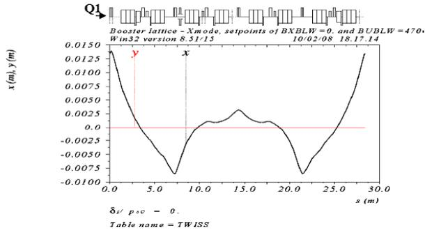
Figure 8: Difference orbit vs. longitudinal position at the operational XMODE with BUBLW=4700 and BXBLW=0.
