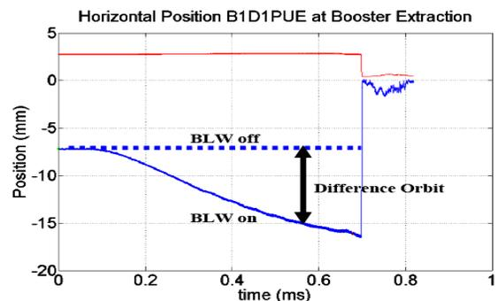
Figure 2: The sum (red) and position (blue) signals of the booster PUEs measured by BEAMTRACK.
