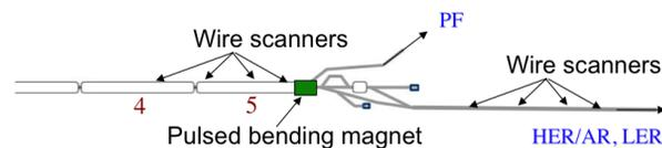
Figure 4: The branching point from the end of LINAC to the BTs for PF, HER/AR and LER. The BT for HER and AR is a common line. Three sets of four wire scanners are installed for optics matching.
