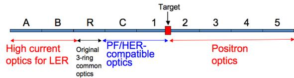
Figure 3: The settings of quadrupole magnets are shown. The horizontal direction shows the axis along LINAC beam line.
