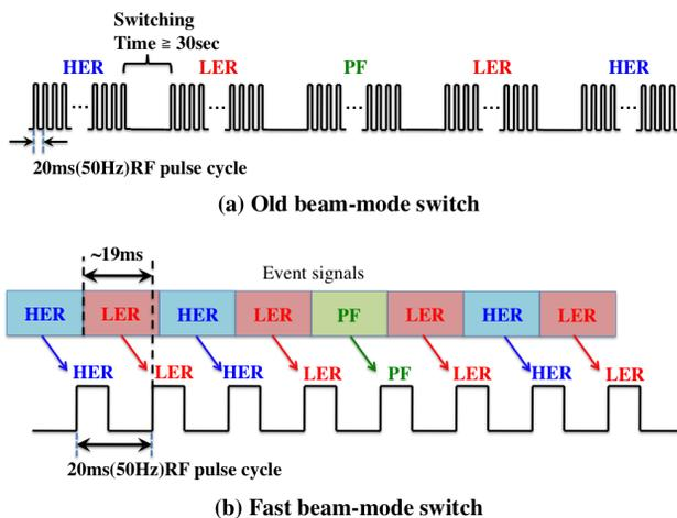
Figure 1: Schematic view of the injection pulses in the two beam-mode switches. The block pulses show beam gate timings. (a) At the slow switch, the beam injection suspended during changing beam-mode. (b) The fast switch tells the next beam-mode 19ms before the beam gate opens.
