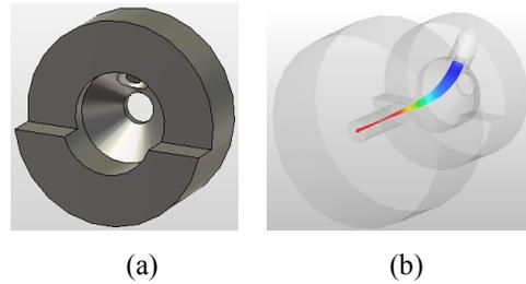
Figure 5: Focusing electrode (a) and beam trajectory (b).
