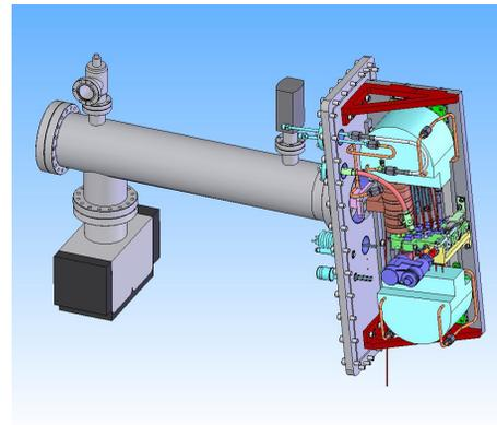
Figure 2: 3D view of the RTM head with open vacuum chamber.
