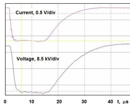
Figure 7: High voltage and current pulses.
