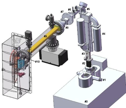
Figure 8: RTM RF system elements.
