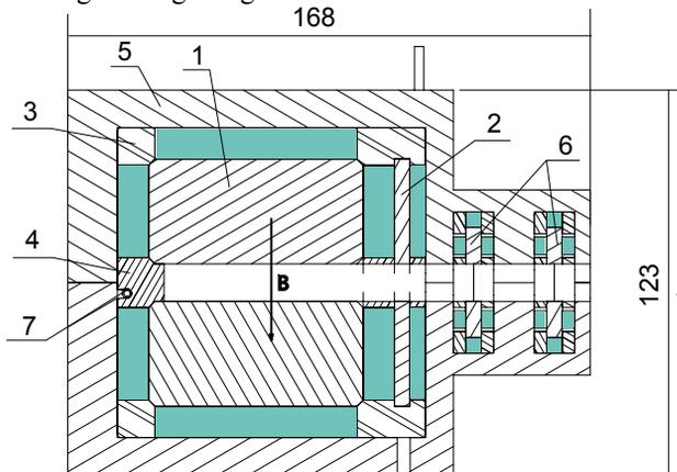
Figure 4: End magnet cross section.
