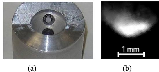
Figure 6: (a) Focusing electrode with the cathode installed, (b) Beam image obtained in prototype tests.
