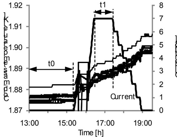
Figure 6: Temperature evolution of a standard sub-sector with normal resistive heating.
