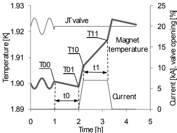
Figure 4: Typical magnet temperature evolution.
