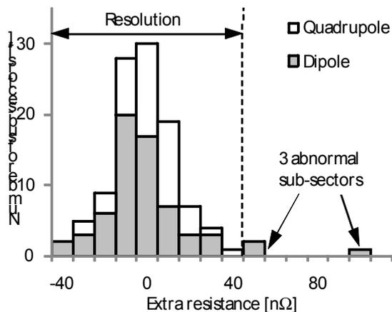
Figure 8: Histogram of extra resistance detected by calorimetry with respect to normal value.
