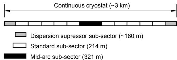
Figure 2: Continuous cryostat sub-sectors.
