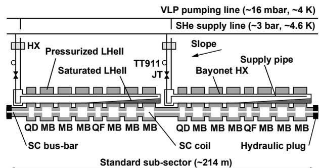
Figure 3: Standard sub-sector cooling loop.
