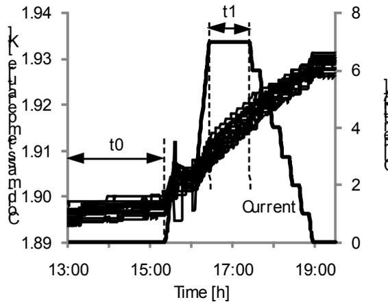
Figure 7: Temperature evolution of a standard sub-sector with abnormal resistive heating.
