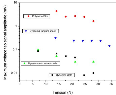
Figure 7: Comparison of maximum voltage tap signal amplitude as a function of tension measured using pen recorder.
