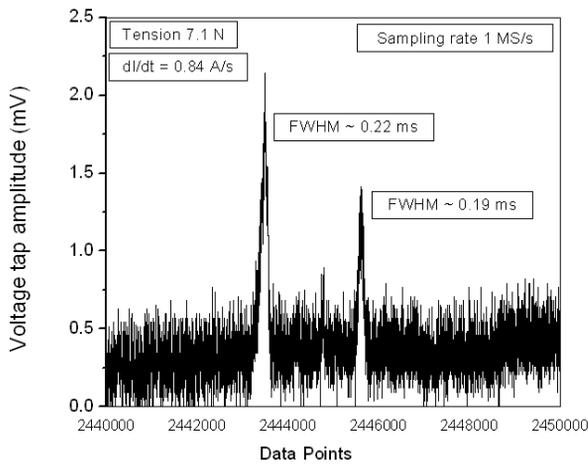
Figure 5: Typical pattern of voltage spike in case of Dyneema cloth.
