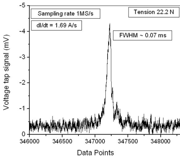
Figure 6: Typical pattern of voltage spike in case of Dyneema random sheet.
