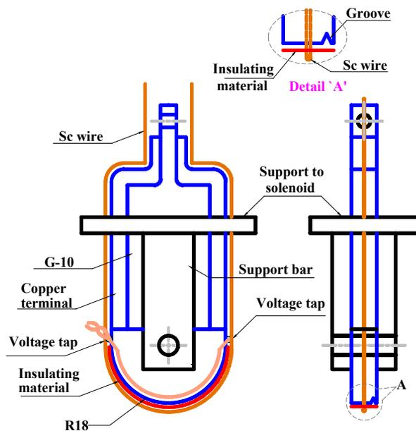
Figure 1: Cross-section of sample holder.
