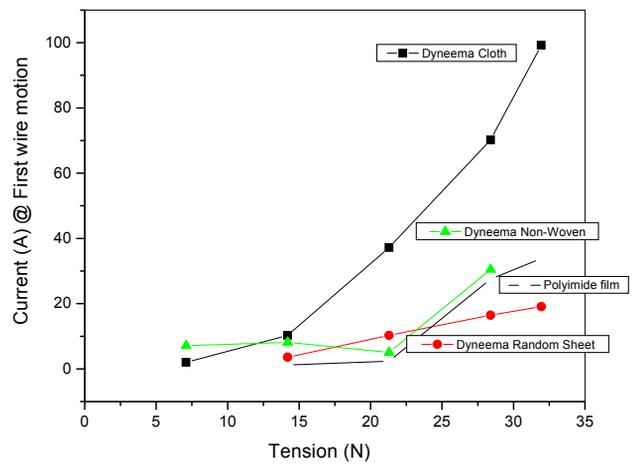
Figure 3: Dependence of current at which wire motion starts as a function of tension.
