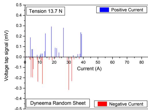
Figure 4: Voltage tap signal after reversing the current polarity in case of Dyneema random sheet measured using pen recorder.
