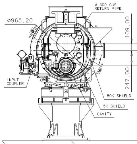
Figure 2: Cross section of Module-C for FNAL cavity.
