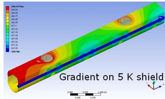
Figure 4: Temperature profile in the 5K shield.
