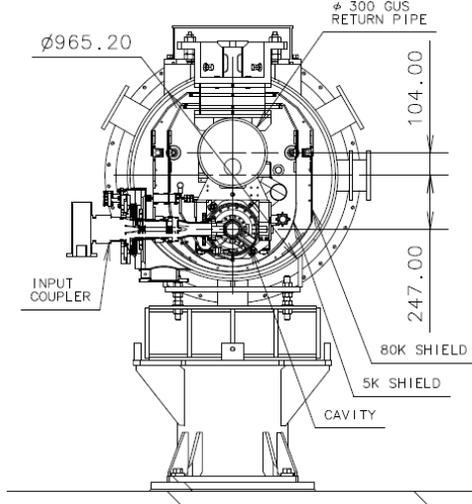
Figure 3: Cross section of Module-A for KEK cavity.
