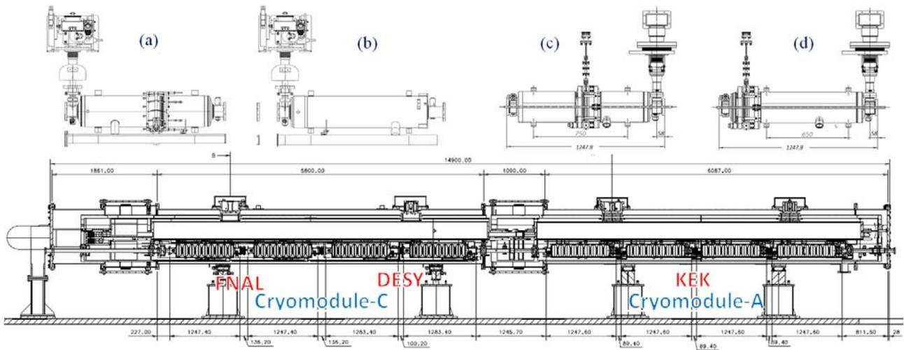
Figure 1: Cross section view of S1-G cryomodule, and the cavity package of each laboratory. (a): FNAL cavity with blade tuner, (b): DESY cavity with Saclay-type tuner, (c): KEK-a cavity with slide jack tuner and (d) KEK-b cavity.
