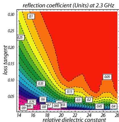
Figure 5: Reflection coefficient simulated with MWS by varying  $\epsilon_r$  and  $\tan \delta$  at 2.3 GHz. Absorber model used is as built for the Ceralloy 137 CA material.
