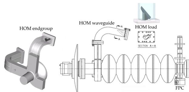
Figure 1: 1497 MHz original CEBAF five-cell cavity design (right) with the HOM absorber layout shown at the top. The HOM endgroup is illustrated separately (left).
