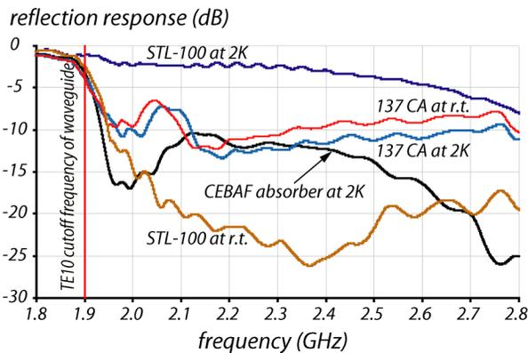
Figure 4: Reflection response of different AlN-based composites measured at room temperature (r.t.) and 2 K.
