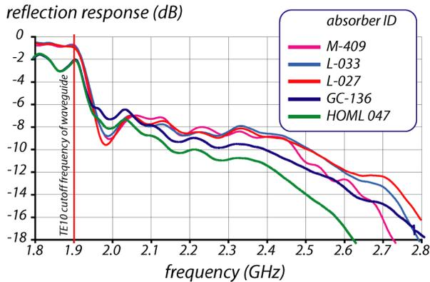
Figure 2: Reflection response of various CEBAF absorbers (glassy carbon AlN ceramic) measured at room temperature. The performance does usually not deteriorate after cool-down to 2K (comp. Figure 4.)
