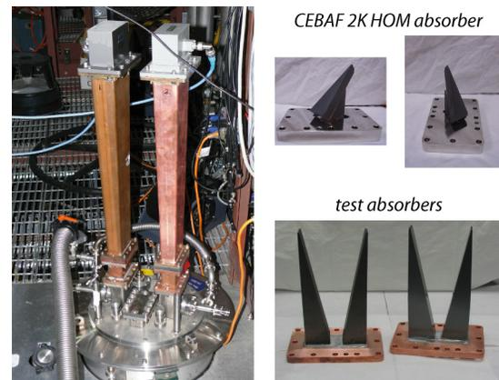
Figure 3: Test setup in the vertical Dewar (left), CEBAF absorber (top right) and two different wedge absorber assemblies (bottom right) made of ceramic AlN-based composites.
