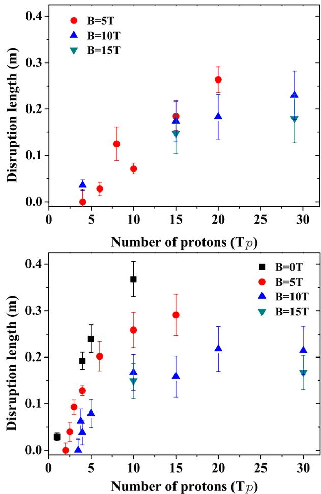
Figure 4: Extent of the proton-beam-induced disruptions: Top: the jet disruptions resulting from a 14-GeV proton beam; Bottom: jet disruptions with a 24-GeV proton beam. In both cases, the proton beam intensity and solenoid magnetic field were varied.
