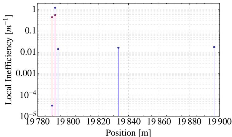
Figure 7: Collimator impact locations for initial distribution in both planes with impact parameter  $1\mu\text{m}$ , comparing MERLIN (with perfectly-absorbing collimators, in red), and SixTrack (with elastic/inelastic and nucleon scattering included, in blue) [12]. Approximate agreement is obtained considering the different physics: primary collimators are impacted
