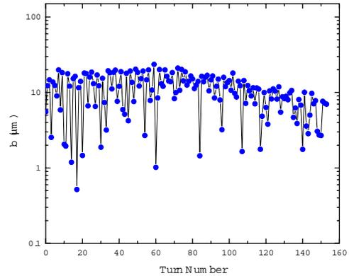
Figure 5: Average impact parameter at TCP.D6L7.B1 as a function of turn number for vertical phase space distribution of  $5.875\sigma$ , into perfectly-absorbing collimator, showing that charge ring is approximately the correct size for collimator simulation.
