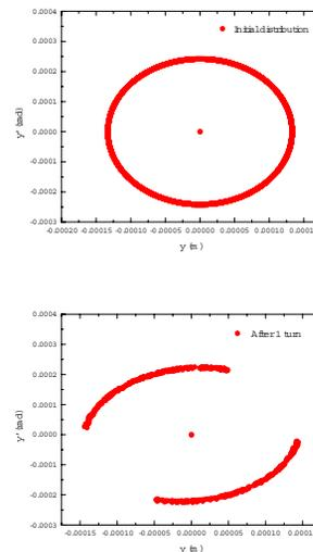
Figure 2: Test of MERLIN code, showing action of primary collimators on a thin ring of particles with distribution in vertical phase space at  $8\sigma$  from the beam centre, with all collimators set to be perfectly absorbing.
