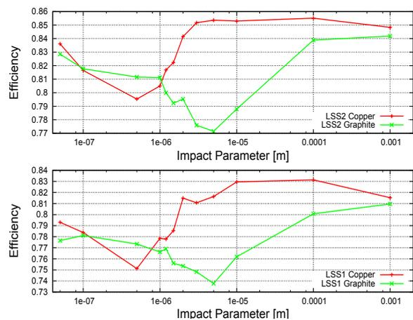
Figure 2: Global efficiency for different impact parameters with collimators in LSS1 (bottom) and in LSS2 (top).
