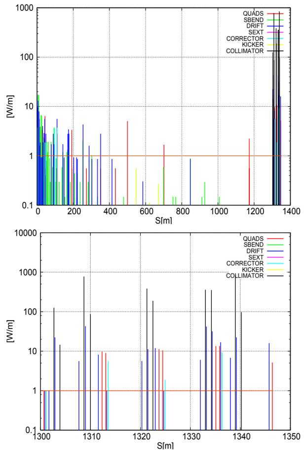
Figure 4: Beam loss maps when collimators are placed in LSS2 (top) and zoom around the collimator section (bottom).
