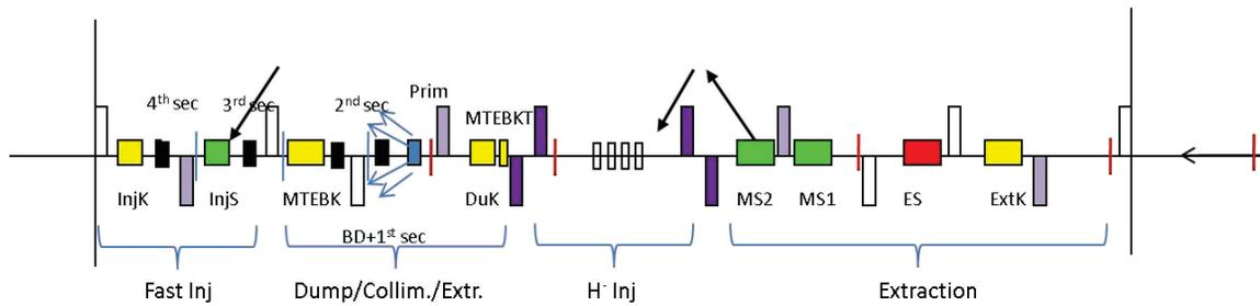
Figure 1: Long straight section layout, including collimators, injection and extraction elements.
