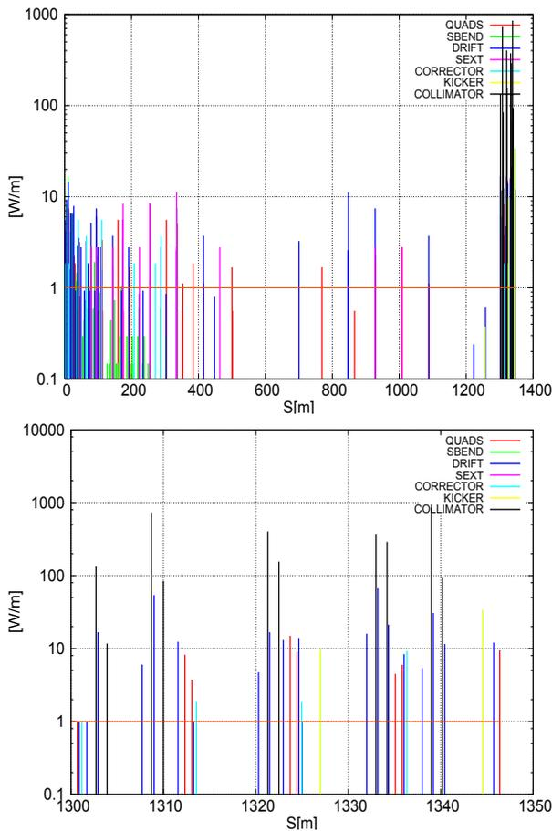
Figure 3: Beam loss maps when collimators are placed in LSS1 (top) and zoom around the collimator section (bottom).
