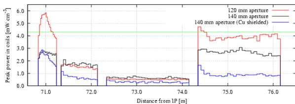
Figure 3: Longitudinal profile of peak power density – for  $L=2.5L_0$  – in the corrector package cables for vertical beam crossing. The red and black curves refer to 120mm (as in the triplet) and 140mm coil aperture, respectively. In the case of the blue curve, a 10mm thick copper liner has been added inside the 140mm coil aperture.
