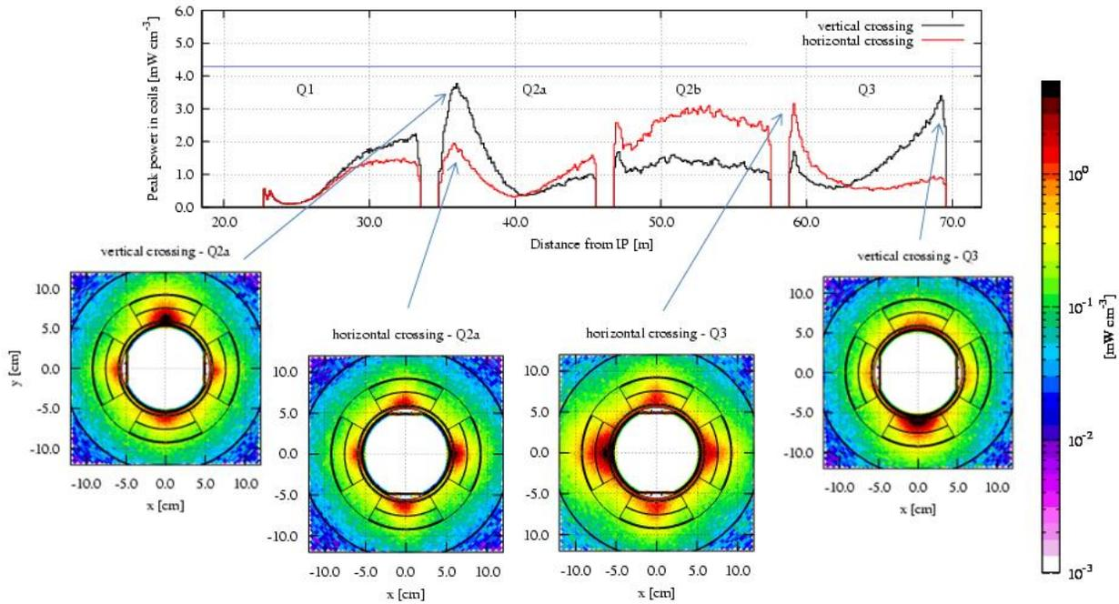
Figure 2: Top frame: Longitudinal profile of peak power density in the quadrupole cables for vertical (black line) and horizontal (red line) beam crossing. Bottom frames: Power density transverse maps at the longitudinal positions corresponding to the maxima indicated by the arrows. The coil aperture is 120mm. Power density values refer to  $2.5 L_0$ .
