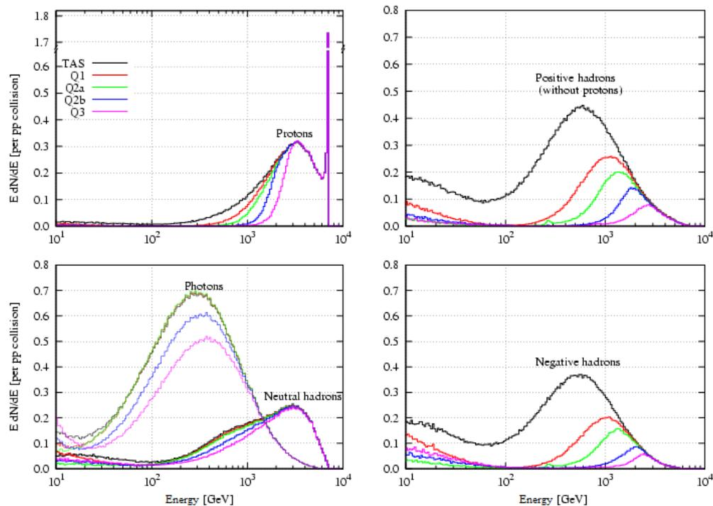
Figure 1: Spectra of particles in the vacuum chamber at the non-IP end of the TAS (black curve) and of each of the triplet quadrupoles (color curves). The four frames refer to different particle families as indicated.
