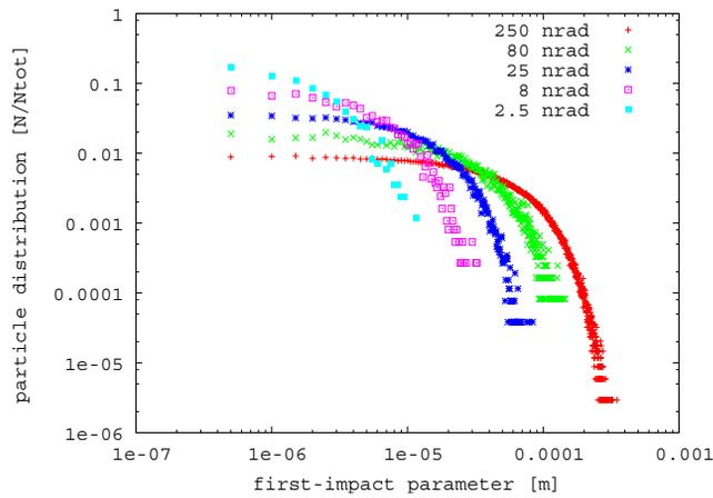
Figure 1: Distribution of the impact parameters of the first impact on the crystal face for diffusive kicks with different maximum amplitudes.
