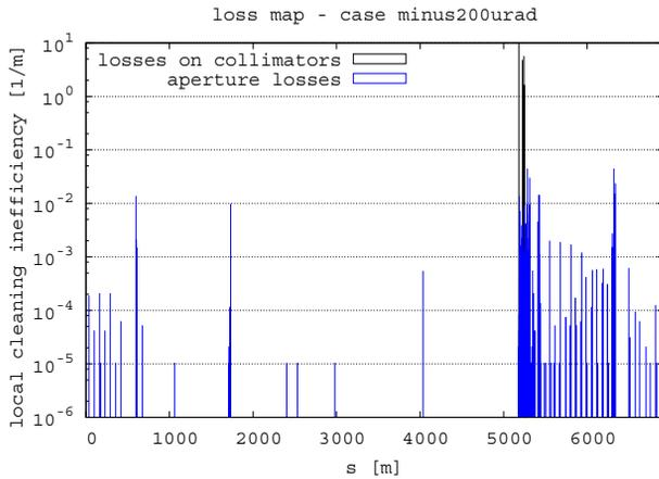
Figure 4: Local cleaning inefficiency along the ring for the crystal in amorphous orientation.
