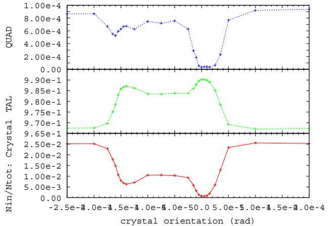
Figure 6: Inelastic interactions at some selected elements (crystal, TAL, QF52210) normalized over the total number of particles absorbed, versus the crystal orientation.
