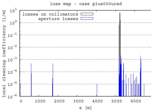
Figure 5: Local cleaning inefficiency along the ring for the crystal in channeling orientation.
