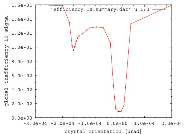
Figure 3: Global cleaning efficiency at  $10\sigma$  for different orientations of the crystal.
