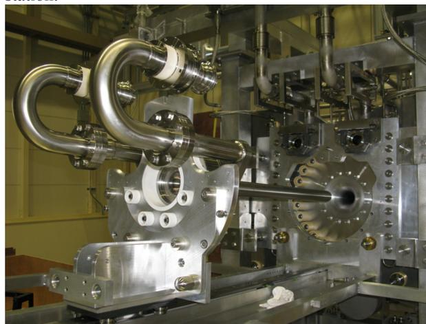
Figure 3: Target assembly being installed in horn.
