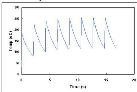
Figure 4: Temperature cycling between pulses at beam centre.
