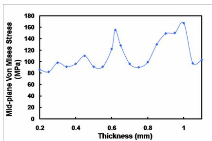
Figure 7: Window max stress with varying thickness.
