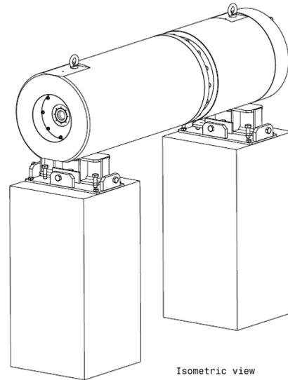
Figure 6: Beam Dump design.
