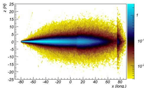
Figure 4: Distribution of the deposited energy in the beam dump, viewed from the top in  $\text{MeV}/\text{cm}^2$ . Normalized to one electron.
