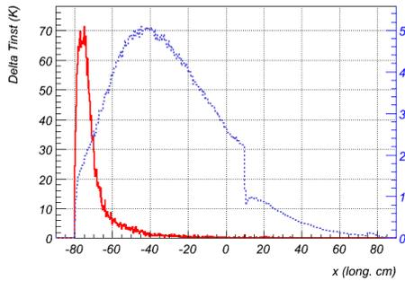
Figure 5: Temperature variation at the dump center ( $r = 0$ ). The two contributions are shown :  $\Delta T_{inst}$  in plain red line with the left hand side axis,  $\Delta T_{eq}$  in dotted blue line with the left hand side axis.
