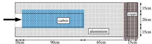
Figure 1: FERMI@elettra Beam Dump design.
