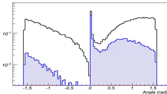
Figure 3: Angular distribution of the secondary particles created in the collimator and exiting it, normalized to 1 electron. The blue dashed histogram is for secondaries with energy above 2 MeV. All particles are included, but neutrons represent less than 1% of the number of particles.
