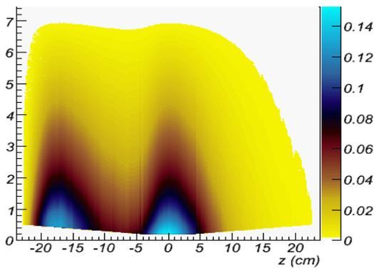
Figure 2: Temperature rise profile in °C for 1 case of halo distribution simulation.
