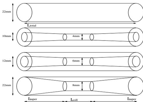
Figure 1: FERMI@elettra collimator design.  $L_{\text{total}} = 45.5$  cm,  $L_{\text{taper}} = 18.5$  cm,  $L_{\text{coll}} = 8.5$  cm.
