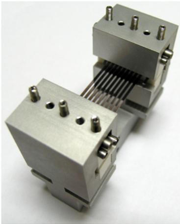
Figure 6: a multi-strip crystal mounted in a bending device.
