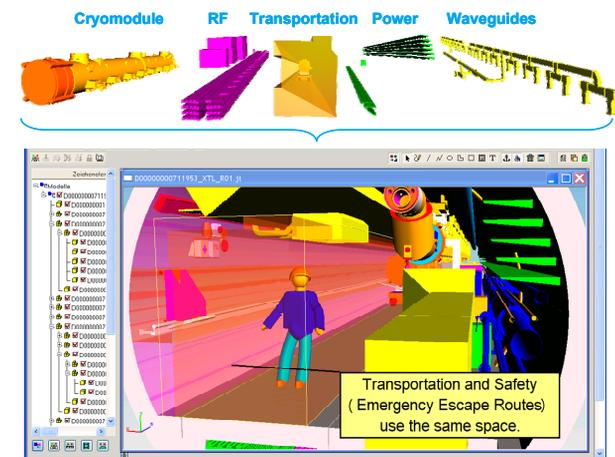
Figure 2: Example for 3D CAD collaboration at XFEL: Work packages are contributing models of their sub-systems in different 3D CAD systems (top), which are then integrated and published in EDMS. The EDMS viewer enables non-CAD-users to access and add reviews to the models (bottom).
