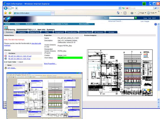
Figure 3: Construction drawing catalogued in EDMS and opened in viewer, enabling multiple reviewers to work in parallel and place mark-ups on the drawing.
