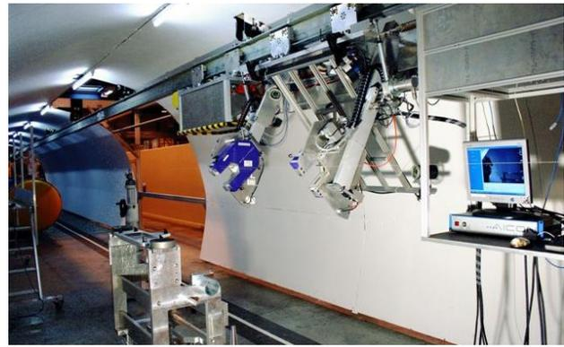
Figure 2: TIM with remote collimator alignment measurement module during testing in tunnel mock-up
