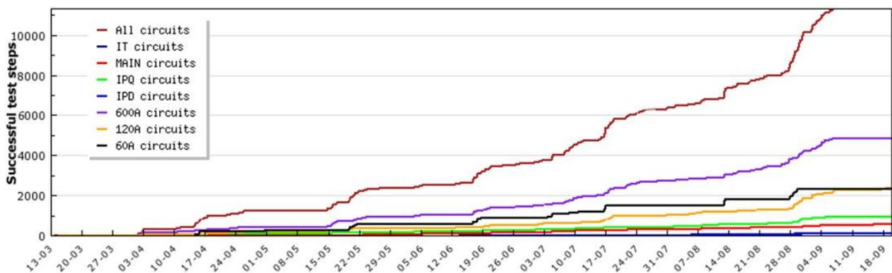
Figure 2: Test step rate during the powering tests of the sc circuit of the LHC in 2008.
