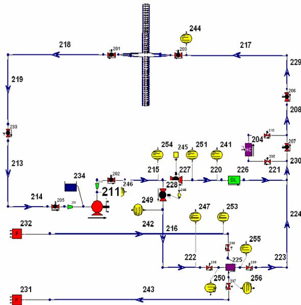
Figure 2: Network model of the pumping skid.
