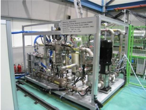
Figure 1: The fabricated water pumping skid in the PEFP
