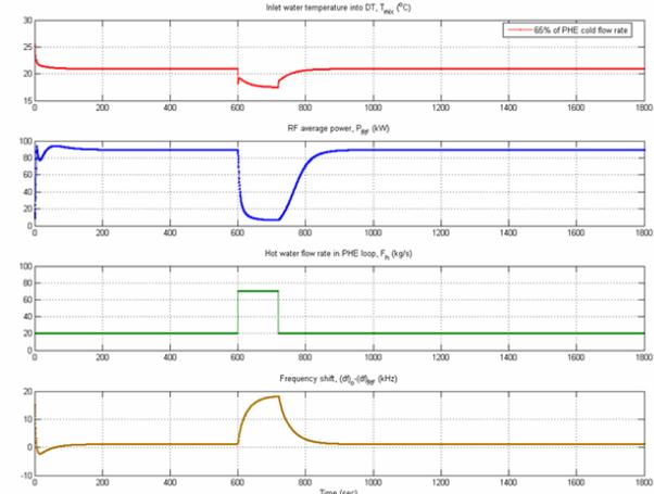
Figure 8: Transient response of frequency shift depending on the temperature variation under various flow rates.
