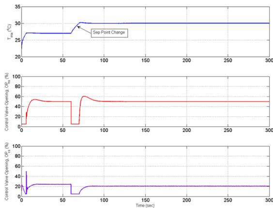
Figure 6: Step up in cooling temperature.
