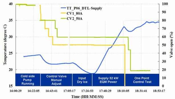
Figure 3: Temperature trend of the DTL supply water during performance test in the PEFP test facility.
