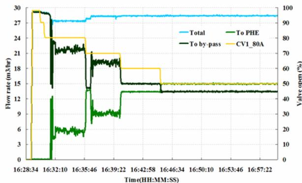
Figure 4: Flow rate balancing in case of valve openings.
