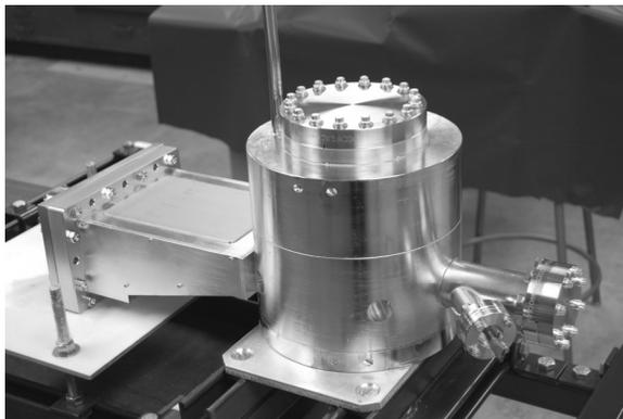
Figure 3: New RF gun after final brazing cycle. Once commissioned, it will be used to generate the high charge drive bunches, using Cesium Telluride photocathodes.
