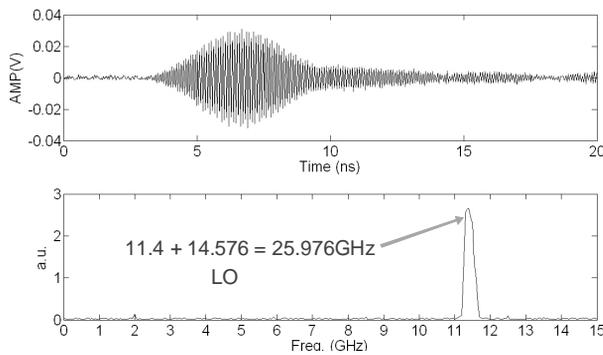
Figure 2: RF pulse extracted from a 26 GHz dielectric loaded wakefield structure, observed on an oscilloscope after its frequency was down converted in a RF mixer (the frequency of the local oscillator was set at 14.576 GHz). Also shown is the FFT of the voltage signal.
