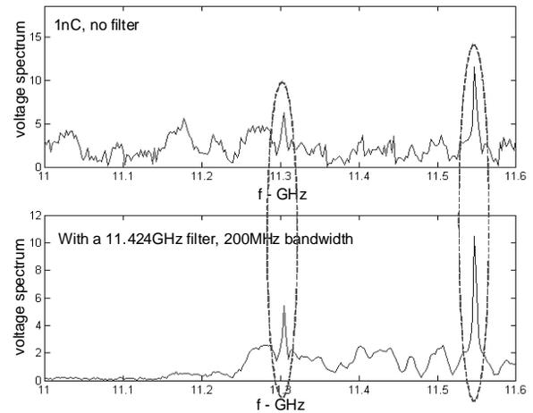
Figure 1: FFT of the antenna signal, used to probe the electric field at the edge of the PBG structure. The plots show the signal without and with a band pass filter.
