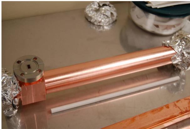
Figure 2: Fabricated 26GHz dielectric-based wakefield power extractor and dielectric (consisting of three 10-cm long dielectric tubes) prior to loading.
