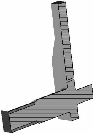
Figure 1: Cross sectional view of the final output coupler design for our proposed 26 GHz dielectric based RF power extractor, modeled using CST Microwave Studio®.
