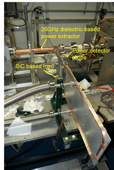
Figure 4: The finished U-shape waveguide, 26GHz RF detector, and SiC based RF load.
