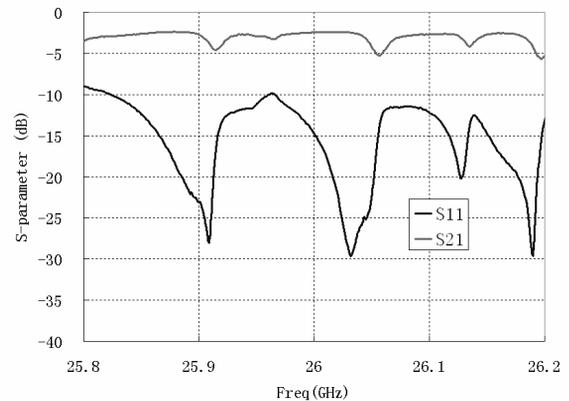
Figure 3: The measured S-parameters of the power extractor.
