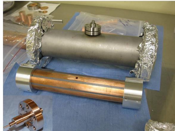
Figure 4: The 7.8GHz transverse mode damped DLA structure and the customized vacuum pipe with a vacuum sealed rf probe.
