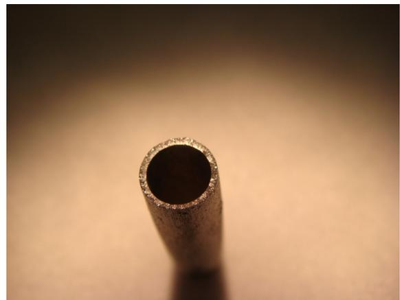
Figure 1. Photograph of CVD diamond tube developed by our collaboration, top view. Tube parameters are: 5 mm inner diameter, 2.5 cm length and ~ 500  $\mu\text{m}$  thick.
