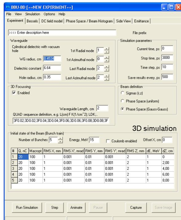
Figure 1. Main screen of the user interface is used for experiment setup definition. Version 2.0 allows specifying 3D beams in Phase Space as upright Twiss ellipses. Uniform and Gaussian initial macroparticle distributions are supported.
