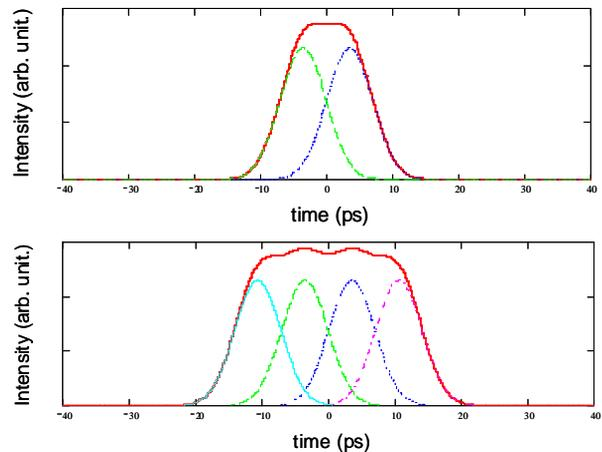
Figure 4. Simulations of two (non-optimized) laser pulse stacking cases for use at the AWA with an a-cut,  $\alpha$ -BBO crystal.
