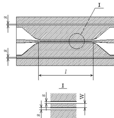
Figure 3: Schematic of a coplanar nonlinear transmission line [11] similar to what is planned for the nonlinear dielectric measurements. Crosshatched areas; copper; open areas: ferroelectric. Dimensions  $s = 20 \mu\text{m}$ ,  $W = 40 \mu\text{m}$ ,  $l = 6 \text{mm}$ .
