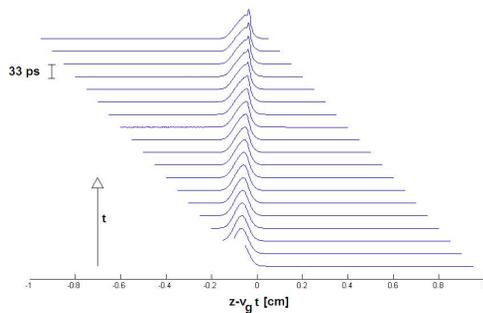
Figure 1: Gaussian pulse traveling down a planar waveguide loaded with a nonlinear dielectric. Note the steepening of the leading edge of the pulse and the growth of the amplitude of the pulse.
