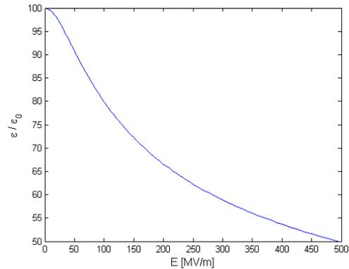
Figure 2: Relative permittivity as a function of electric field strength for a composite ferroelectric dielectric [4].
