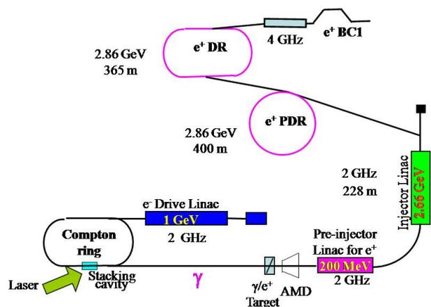
Figure 1: CLIC Injector Complex with Compton Ring
