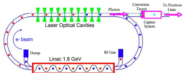
Figure 3: Basic layout for an ERL scheme
