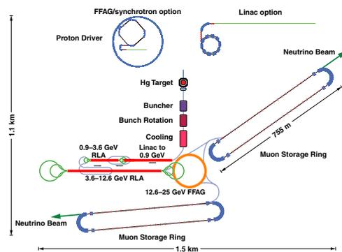
Figure 1: Schematic layout of the baseline accelerator facility that is being developed within the International Design Study for the Neutrino Factory [2].
